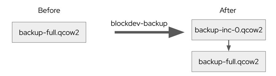
Given an existing full backup and dirty bitmap tracking, blockdev-backup can copy out changed blocks into a new qcow2 file.
